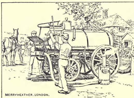
Fig. 9. Merryweather's Cesspool Emptier with Deodorising Stove.
